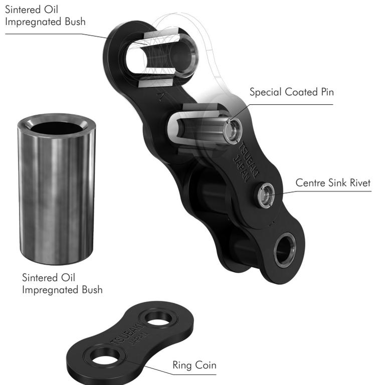
Fig. 10 Basic Construction
