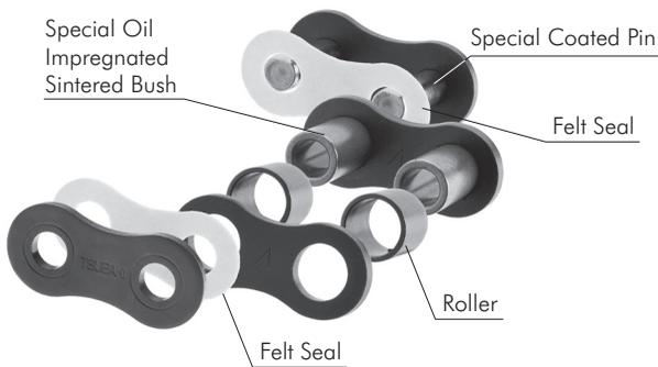
Fig. 11 Basic Construction
