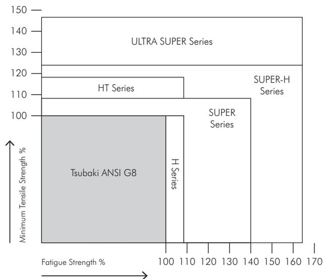
Fig. 16 Comparison of Tensile Strength / Fatigue Strength
